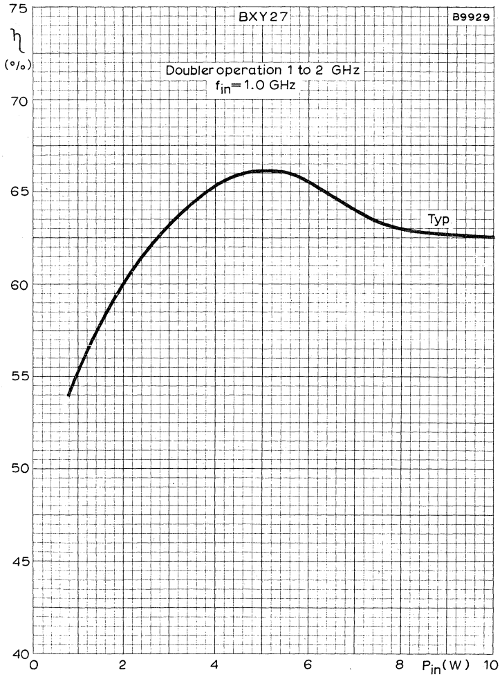
OVERALL EFFICIENCY PLOTTED AGAINST INPUT POWER FOR DOUBLER OPERATION
